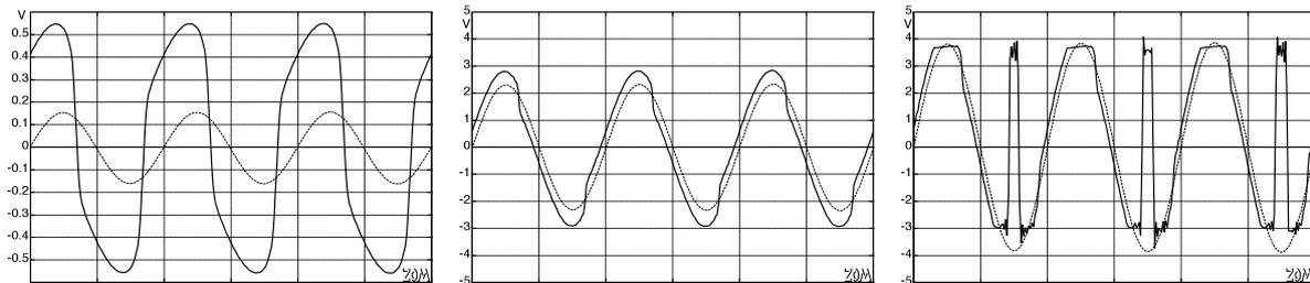
**Fig. 10.8.35:** Time function for different drive-levels ( $f = 500$  Hz).  $U_{\text{Batt}} = 9$  V.
