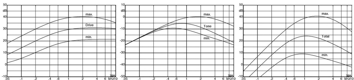
**Fig. 10.8.36:** Tube-Screamer-frequency responses: distortion unit, sound filter. Overall circuit. The transfer function of the sound filter is easily calculated by Y-delta-transforming the OP-amp input circuit.
