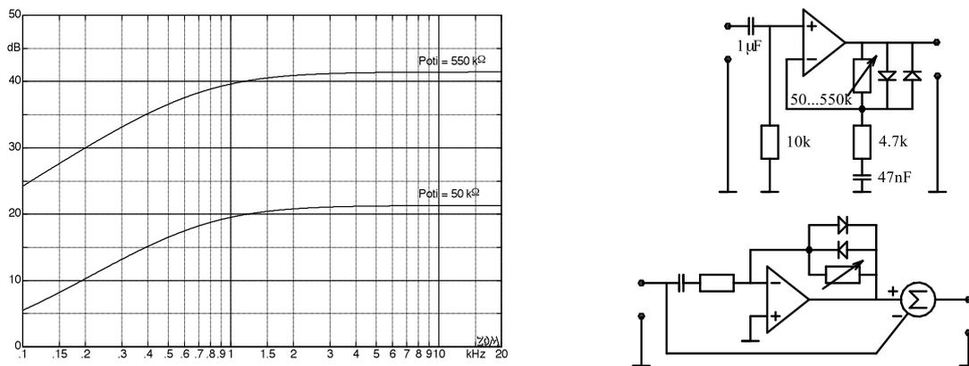
**Fig. 10.8.34:** Tube-Screamer: small-signal frequency-response and schematic of the distortion section.
