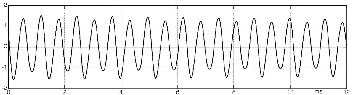
**Fig. 11.70:** Time function of sound pressure in a sub-harmonically distorted sinusoidal tone:  $f = 1,6 \text{ kHz}$ .
