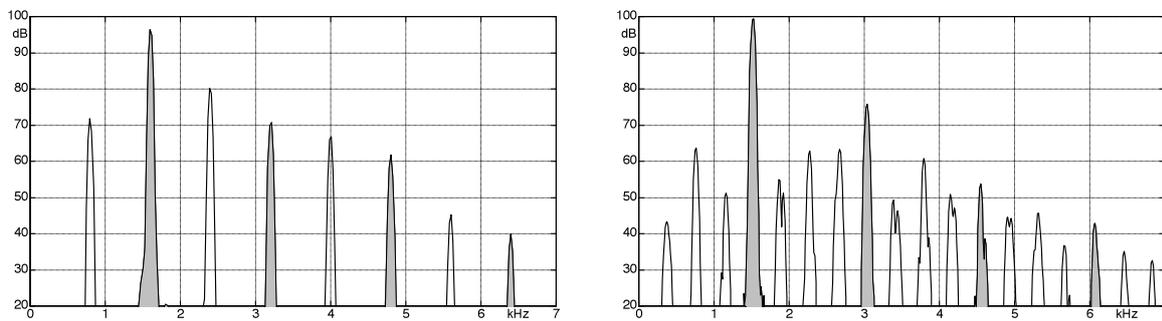
**Fig. 11.68:** Sub-harmonics at half (left), and a quarter (right) of the excitation frequency.
