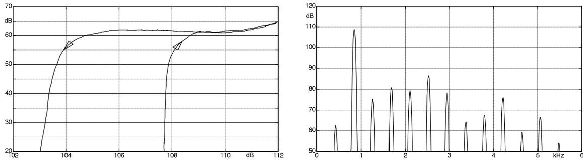
**Fig. 11.72:** Level-hysteresis (left), distortion spectrum (right). Celestion Vintage-30,  $f = 844$  Hz.
