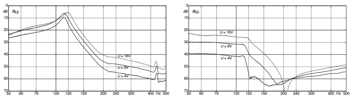
**Fig. 11.65:** Frequency-dependence of harmonic distortion in the current when fed from a stiff voltage source (as in Fig. 11.64). The drive-level-dependent shift of the maximum is a result of the strong non-linearity.
