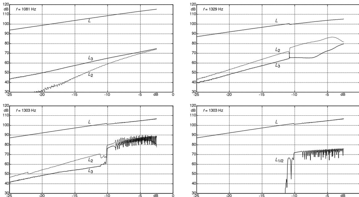
**Fig. 11.73:** Sum SPL  $L$  and distortion level, Eminence L-105; 0dB = maximum power. Lower left: for  $f = 1303$  Hz, the level development of the sub-harmonic ( $f/2$ ) is shown.
