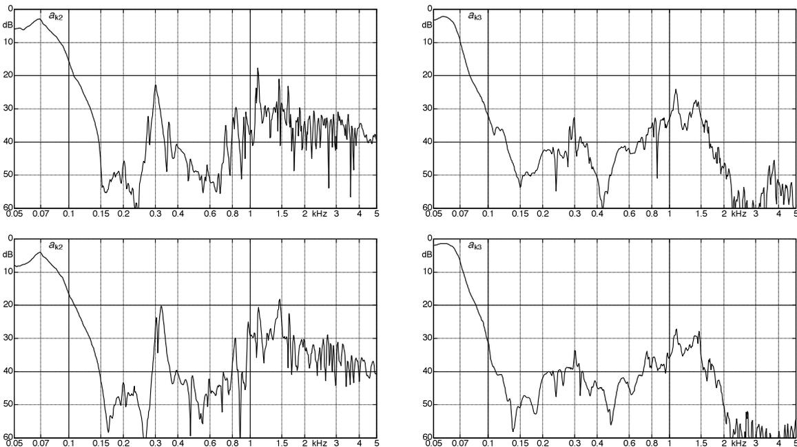
Fig. 11.67: 2<sup>nd</sup>- and 3<sup>rd</sup>-order distortion. Enclosure: VOX AD-60VT,  $U = 10V$ ,  $d = 3m$ .
