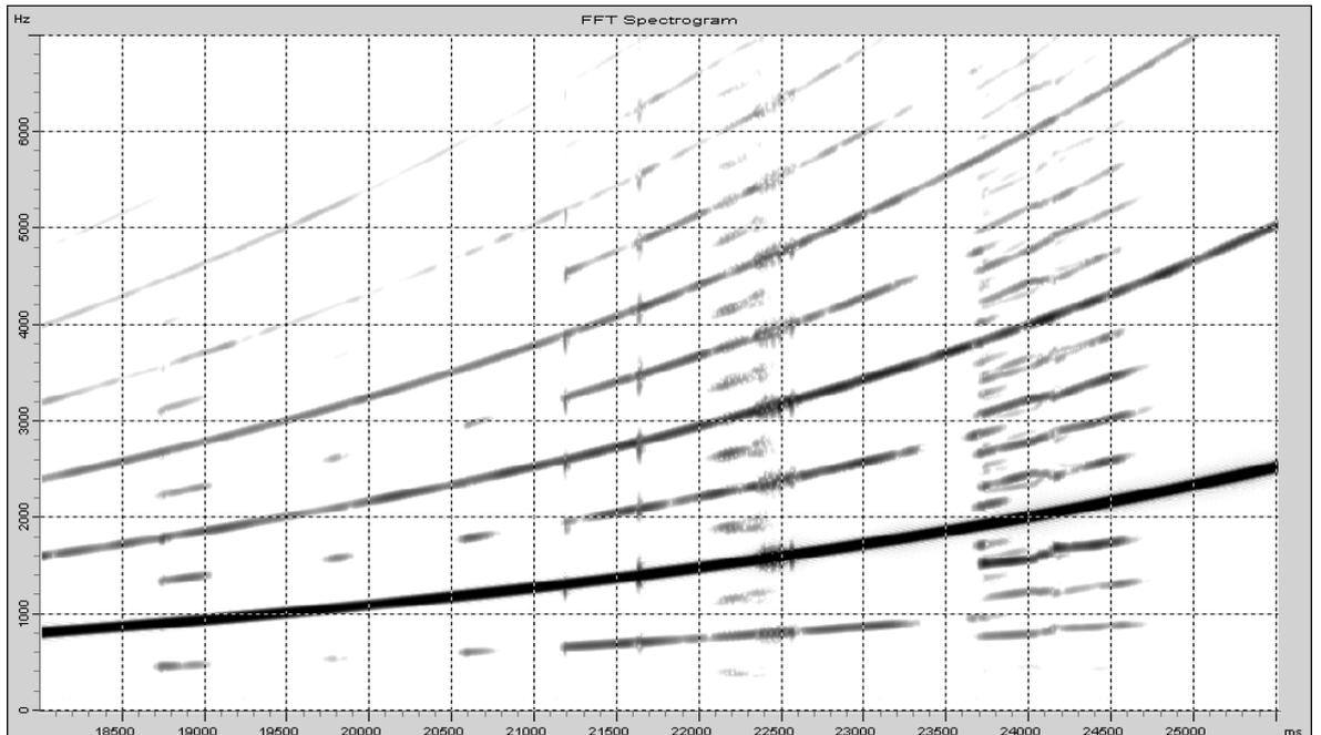
**Fig. 11.71:** Jensen P12-R, sweep-spectrogram,  $f = 800 - 2500 \text{ Hz}$ ,  $U = 10 \text{ V}$ .
