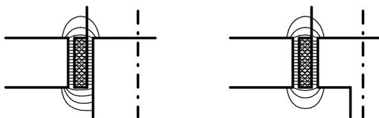
**Fig. 11.63:** Different designs of the pole-core. On the left it is purely cylindrical, on the right offset. The scatter-field generated outside of the air gap depends on the geometry of the pole-core.
