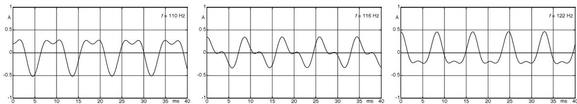
**Fig. 11.64:** Time-functions of the loudspeaker-current fed from a stiff voltage source,  $U = 10\text{V}$ ; VOX AD60-VT.
