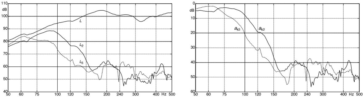
Fig. 11.66: Frequency responses of SPL (left) und distortion level. VOX AD60-VT,  $U = 10V$ .
