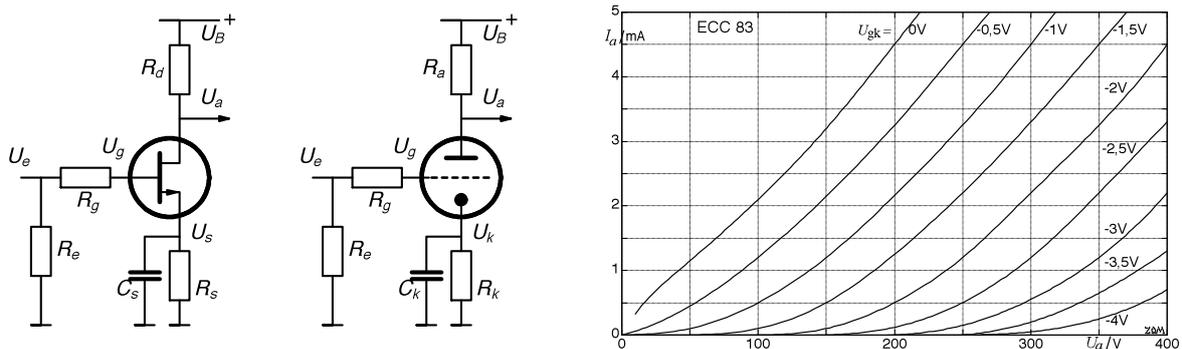
**Fig. 10.1.1:** Input-circuit of a tube amplifier (center) compared to a FET-amplifier (left). The right-hand picture shows typical characteristics (data-sheet of the double-triode-tube ECC83). The term “control voltage” is used in various ways – here, the grid/cathode-voltage and the gate/source-voltage is meant.
