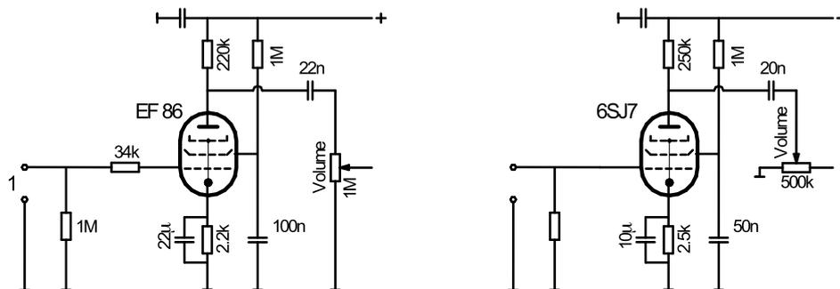
**Fig. 10.1.31:** Pentode-input-stages in guitar amplifiers: VOX AC-15 (left), Fender Dual Professional (right).
