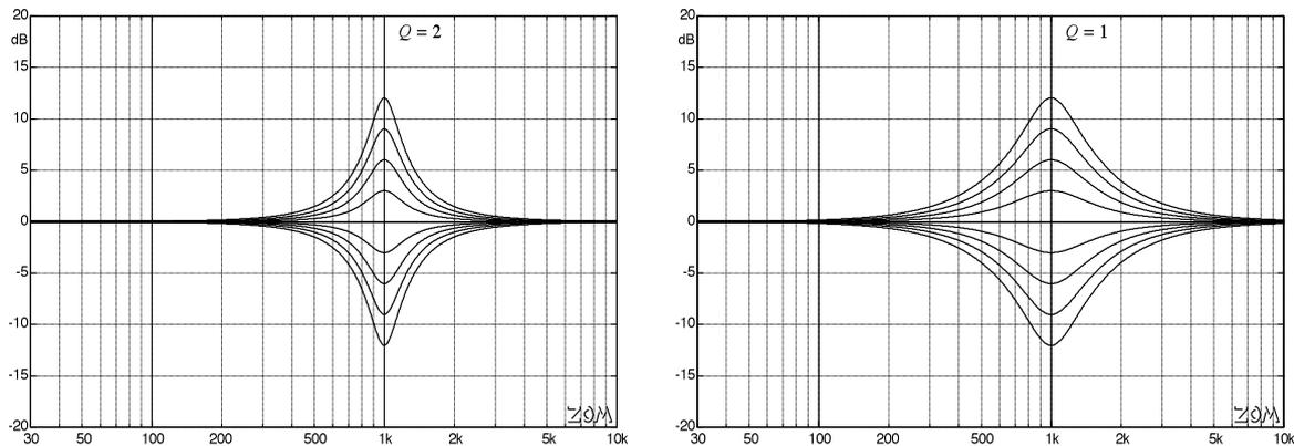
**Fig. 10.3.17:** Equalizer characteristic.  $B = 20 \cdot \lg(\beta) = [-12 \ -9 \ -6 \ -3 \ 0 \ 3 \ 6 \ 9 \ 12]\text{dB}$ ,  $f_x = 1 \text{ kHz}$ .
