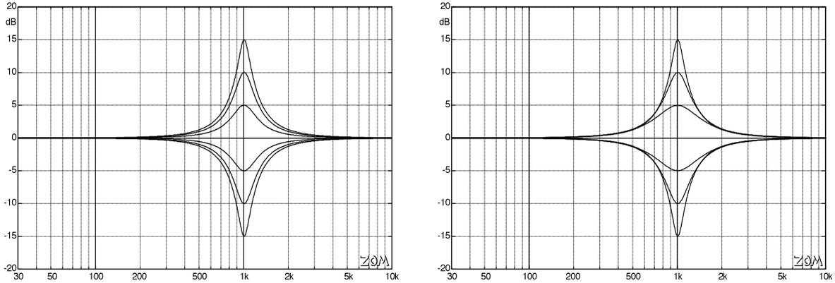
**Fig. 10.3.21:** Transmission characteristics of the EQ-circuit according to Fig. 10.3.20.
