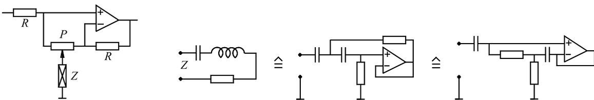
**Fig. 10.3.20:** Active EQ-circuit. The series-resonance-circuit ( $Z$ ) may be realized via either active circuit. The active resonant circuits are approximations of an ideal series-resonance circuit
