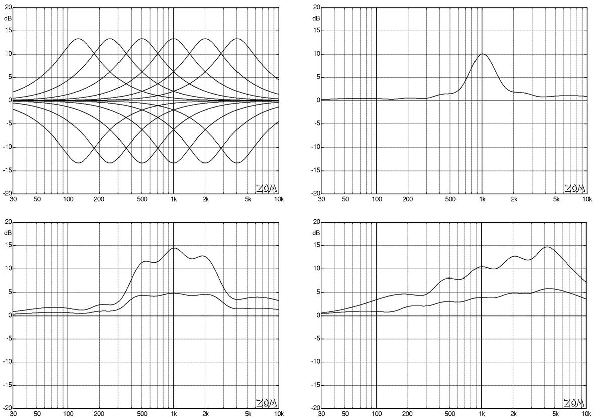
**Fig. 10.3.22:** Octave-equalizer: single filter (upper left). Six-band EQ, boost only in the 1-kHz-channel (u. right). Boost only in 3 bands (lower left). Boost increasing with frequency (l. right).
