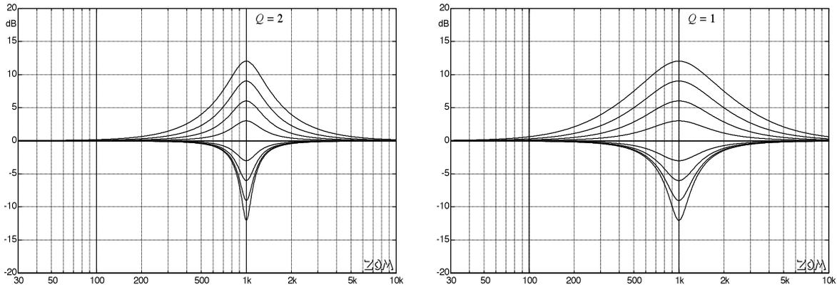
**Fig. 10.3.18:** Characteristic of a Constant- $Q$ -Equalizer. The specified  $Q$  is the denominator- $Q$ .
