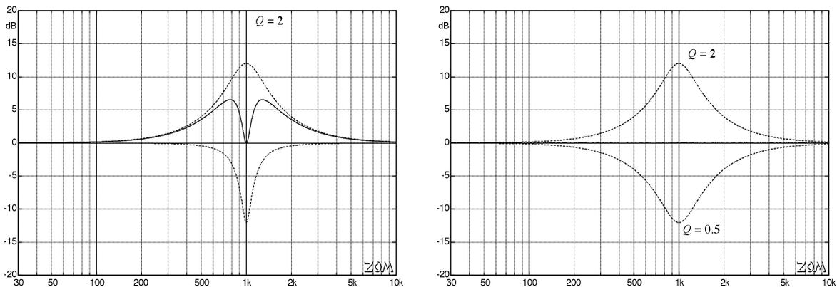
**Fig. 10.3.19:** Series-connection of two constant- $Q$ -equalizers. Single filter (----) and series connection (—). For the gain to add up to 0, both  $Q$ -factors need to be reciprocal (right-hand picture).
