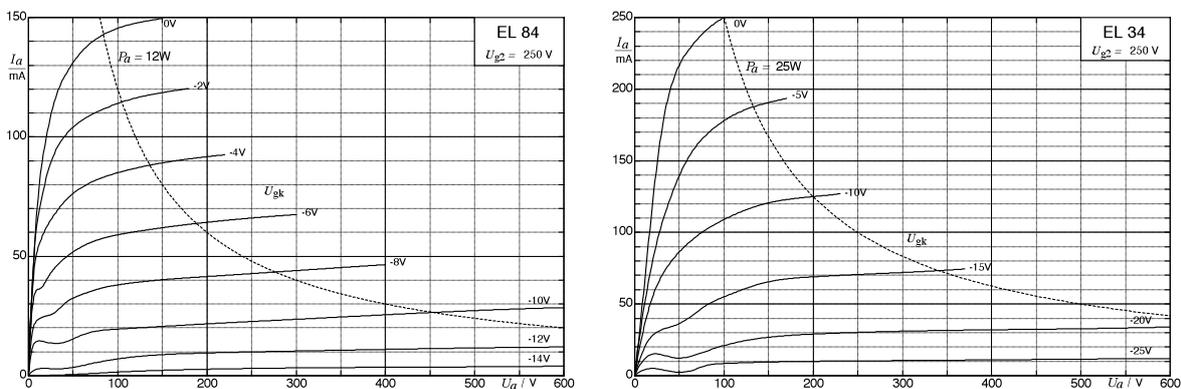
**Fig. 10.5.1:** Family of output characteristics of two typical power-pentodes. Screen-grid-voltage  $U_{g2} = 250\text{V}$ .
