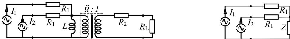
Fig. 10.5.14: The rigidly-coupled output transformer as three-port. Right: simplified circuitry;  $\dot{i} = TR$ .
