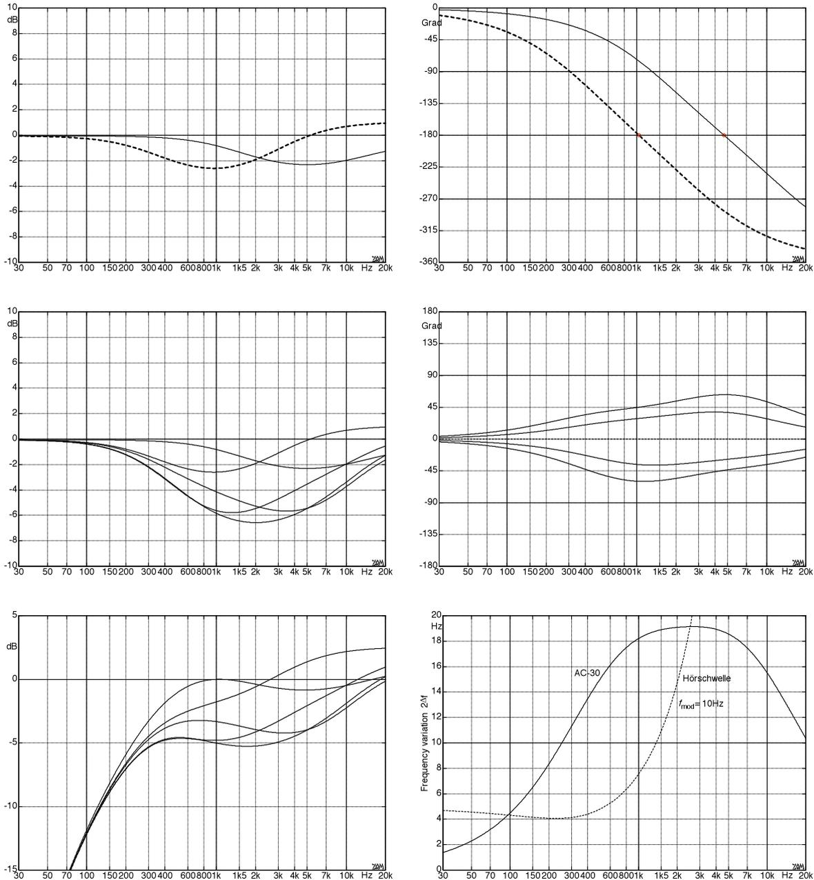
**Fig. 10.8.16:** AC-30-modulator. Top: magnitude and phase characteristic of both all-pass filters. Middle: Magnitude- and normalized phase characteristic of the overall modulator. Bottom: Magnitude characteristic incl. 4<sup>th</sup>-order high-pass; frequency change  $2 \cdot \Delta f$  achievable with  $f_{LFO} = 10\text{Hz}$ . “Hörschwelle  $f_{mod}=10\text{Hz}$ ”: threshold for just noticeable FM at a modulation frequency of 10 Hz
