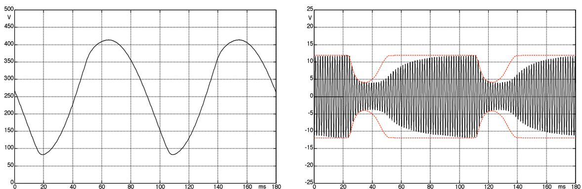
**Fig. 10.8.13:** LDR-modulator. LFO-signal at the plate of the oscillator-tube (left), 600-Hz-sine-tine modulated by the LDR (right). Dashed: imaginary effect of a modulator with zero recovery time.
