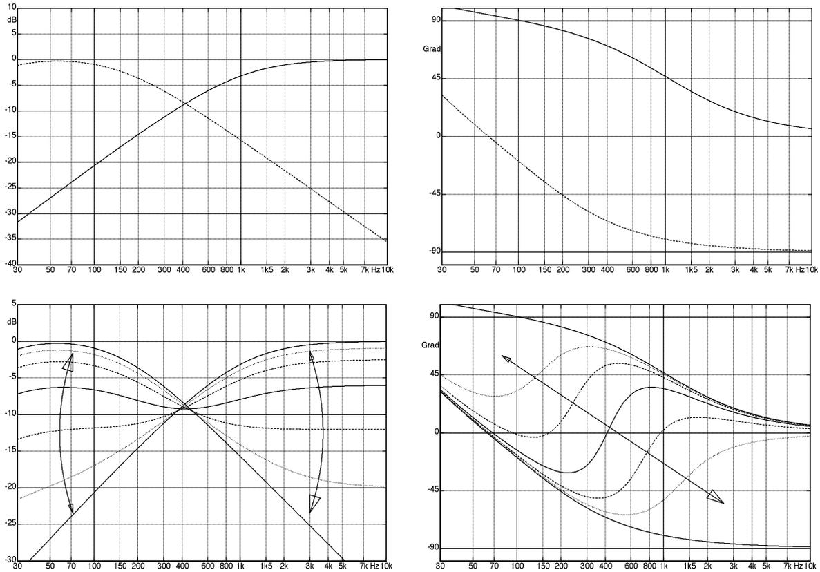
**Fig. 10.8.14:** Magnitude- and phase-characteristics of the frequency crossover (top), and of the overall system (bottom). 5G13.
