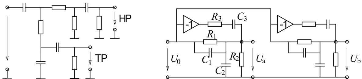
**Fig. 10.8.15:** Frequency crossover of the Vibrasonic 5G13 (Fender, left), and of the AC-30 (VOX, right).
