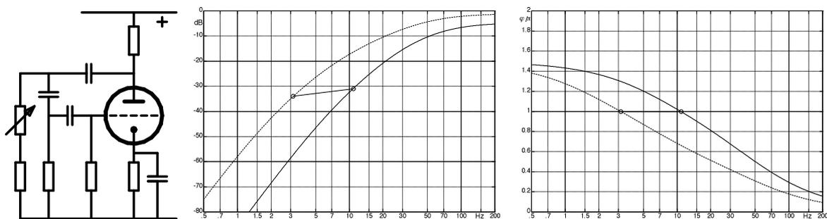
**Fig. 10.8.12:** LFO-circuit in a tube amplifier; magnitude- and phase- characteristics of the feedback network.
