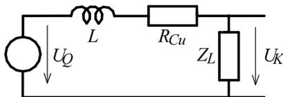
**Fig. 4.36:** Equivalent circuit of the coil with inductor  $L$  and resistance of the copper wire  $R_{Cu}$ .
