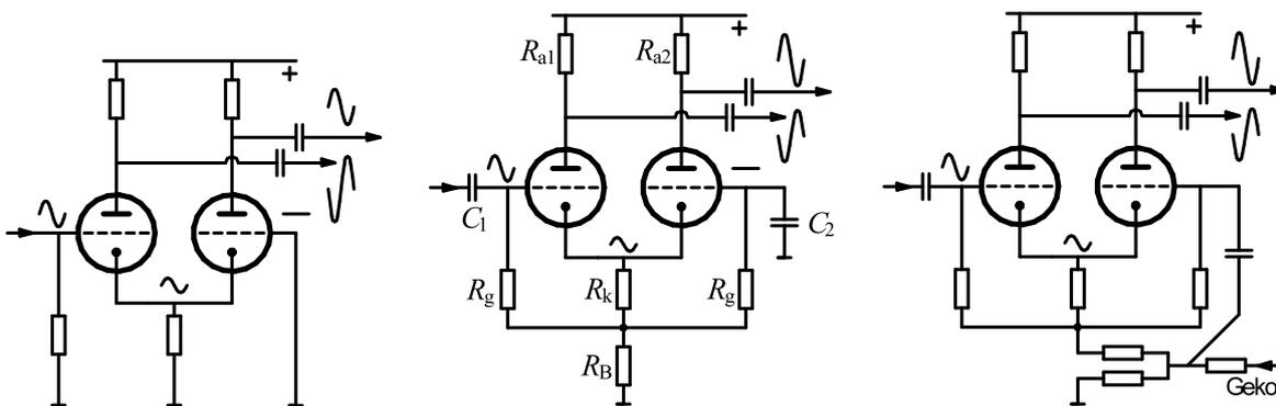
**Fig. 10.4.8:** Differential amplifier with negative feedback via the cathode (Geko = negative feedback).
