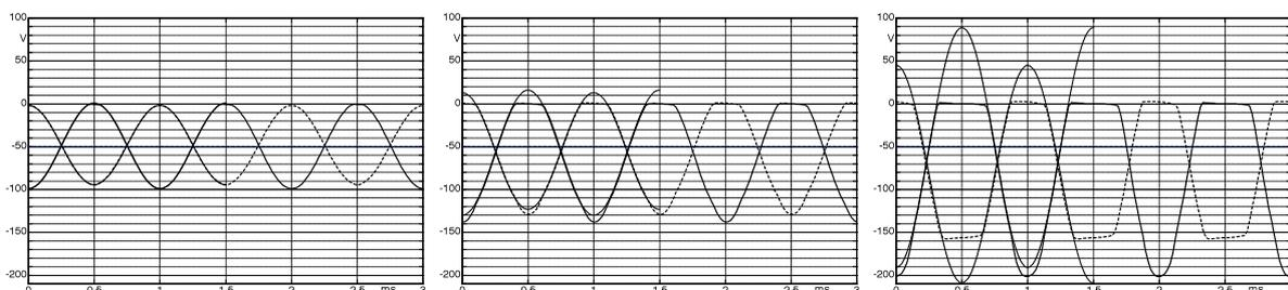
**Fig. 10.4.9:** Measurements at the differential amp of a Fender Super-Reverb (AB-763, negative feedback deactivated). Power-tube bias =  $-50\text{ V}$ . Grid-voltage of the 1<sup>st</sup> power tube ( $V_7 = \text{—}$ ), and of the 2<sup>nd</sup> power tube ( $V_8 = \text{---}$ ). On the left, undistorted cosine-oscillations are shown for comparison.
