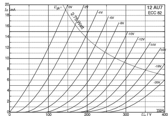
Fig. 10.11.1: Output characteristics of triodes (according to data sheets).
