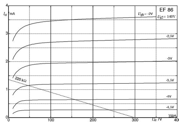
Fig. 10.11.2b: Pentode-characteristics for comparison: left Telefunken, right Svetlana.
