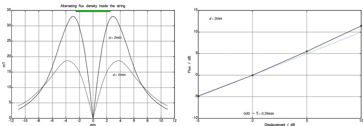
**Fig. 5.4.17:** String-internal axial alternating flux-density (RMS value). The diameter of the cylindrical magnet is marked in grey. On the right the normalized drive-dependency of the alternating flux density.
