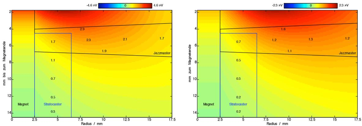
**Fig. 5.4.15:** alternating voltage in the winding dependent on the number of turns and the distance to the pole plate. The coil cross-sections marked are those for Stratocaster- and Jazzmaster-pickups. On the left, the distance between string and magnet is 2 mm, on the right it is 4 mm. The numbers entered in the figure have the dimension  $\mu\text{V} / \text{turn}$ .
