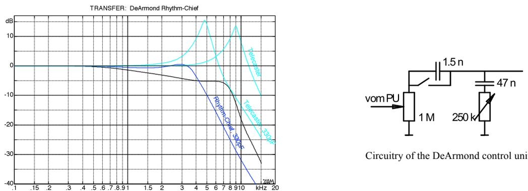
**Fig. 5.4.47:** transfer frequency response for the Rhythm-Chief 1100; Telecaster Bridge-pickup fro comparison.
