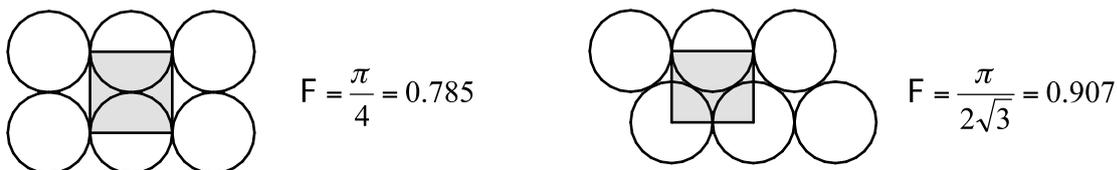
**Fig. 5.5.2:** Fill factor  $F$  for ideal wire positioning. The cross-section of the copper itself is – for a wire with a single layer of varnish – approx. 80% of the full wire cross-section area; for a double layer of varnish approx. 70%. Depending on manufacturer, insulation type and manufacturing method other values may result!
