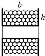
**Fig. 5.5.1:** Cross-section through a pickup coil. Winding width  $b$  and winding height  $h$  define the interior dimensions of the bobbin. The wire diameter is shown drastically enlarged.
