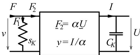
**Fig. 6.1:** Equivalent circuit of the piezo-transducer. The driving force  $\underline{F}$  is divided up into  $\underline{F}_1$  and  $\underline{F}_2$ .
