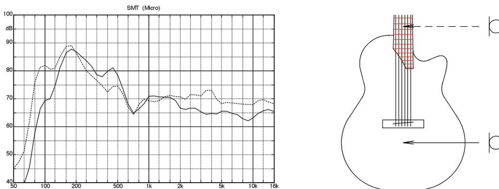
**Fig. 6.24:** Measured  $1/3^{\text{rd}}$ -octave spectra (SPL re.  $20 \mu\text{Pa}$ ) and microphone positions (at 12 cm distance). Arbitrarily fingered chords, strings struck with a pick in quick succession. “Mikro“ = microphone (“mike”), “Frequenz” = frequency.
