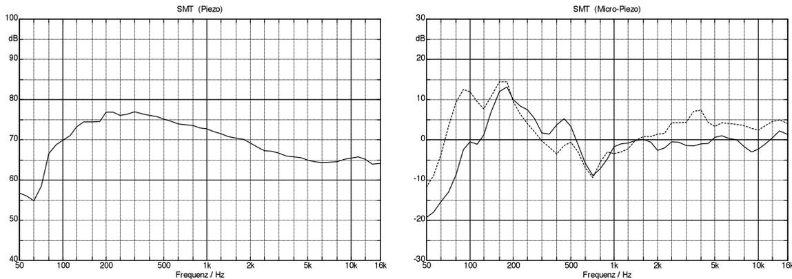
**Fig. 6.25:**  $1/3^{\text{rd}}$ -octave spectra of the piezo signal (left); 0 dB arbitrarily set for a curve comparable to the one in Fig. 6.24. Right: difference “mike-spectrum minus piezo-spectrum” (2 mike positions). “Micro” = mike
