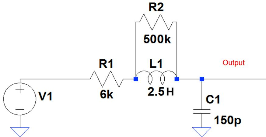
**Fig. 2:** Electrical equivalent circuit of the Stratocaster pickup; V1 is the electrical voltage induced by the vibrating string.
