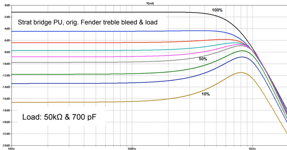
**Fig. 11:** Low-impedance load; frequency responses of the Fender recommended treble-bleed arrangement (1000 pF in parallel with 150 k $\Omega$ ), at various positions of the volume control in % of the full turn angle.
