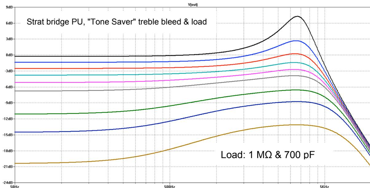
**Fig. 12:** Frequency responses of the second Fender recommended treble-bleed arrangement ("Fender Tone Saver"; 1000 pF in series with 130 kΩ), at various positions of the volume control in % of the full turn angle.
