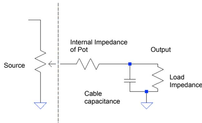
**Fig. 5:** Equivalent circuit of volume control, cable and input impedance of amplifying device.
