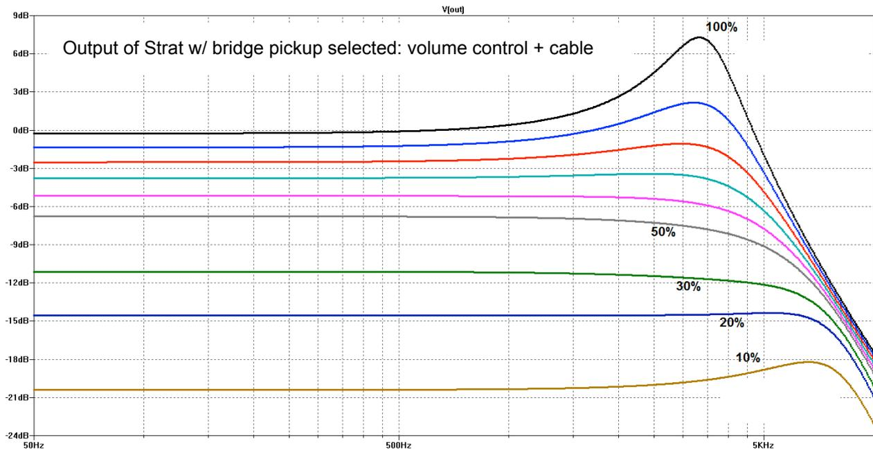
**Fig. 8:** Overall frequency response at the output of the guitar with cable attached; parameter is the position of the volume control in % of the full turn angle.
