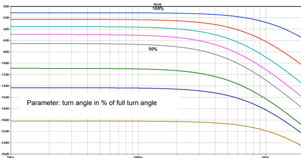
**Fig. 6:** Frequency response of the low-pass formed by volume control and cable capacitance; for various settings of the turn angle.
