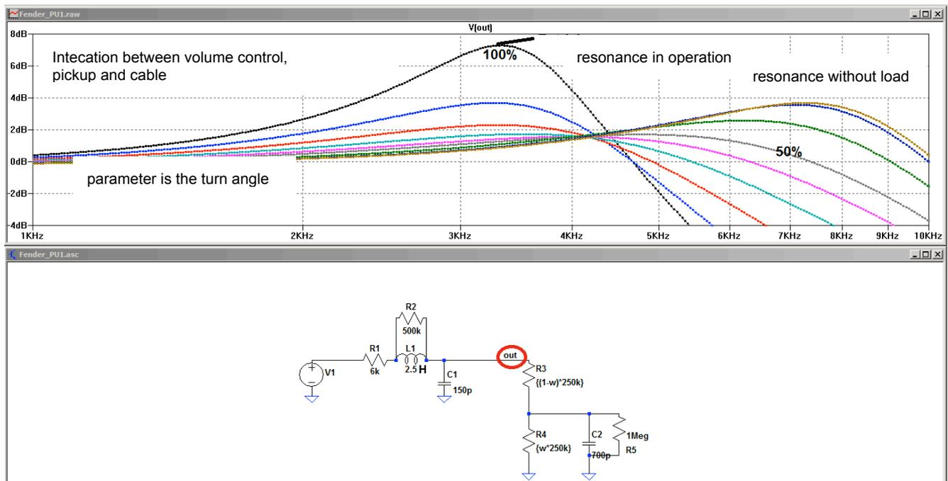
**Fig. 7:** Interaction between volume control, pickup, and cable. Top: frequency response of the system at the output of the pickup. Parameter is the position of the volume control in % of the full turn angle.
