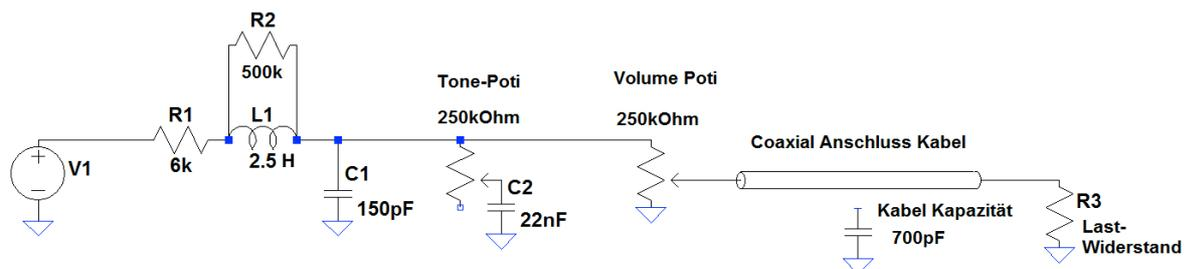
**Fig. 4:** Complete equivalent circuit for the Stratocaster, neck or middle pickup selected
