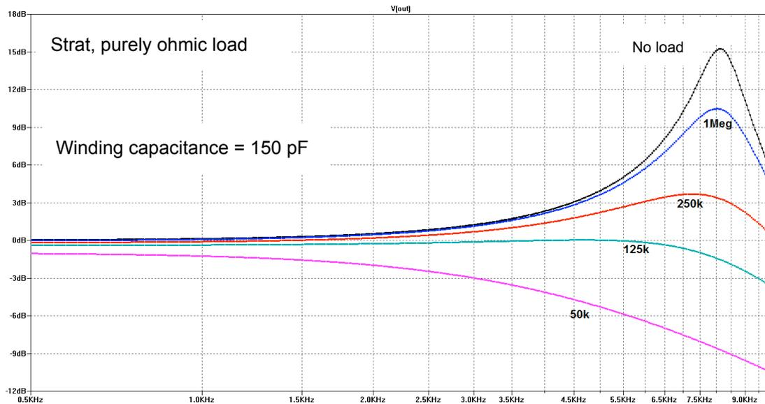
**Fig. 3:** Resonance behavior of the Stratocaster pickup with purely ohmic load
