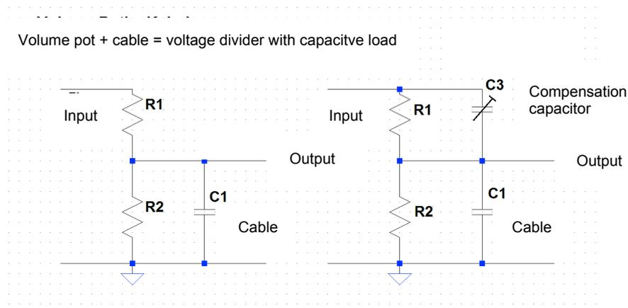
**Fig. 9:** Equivalent circuits of Strat volume control without (left) and with (right) compensation capacitor – here shown as an adjustable cap.
