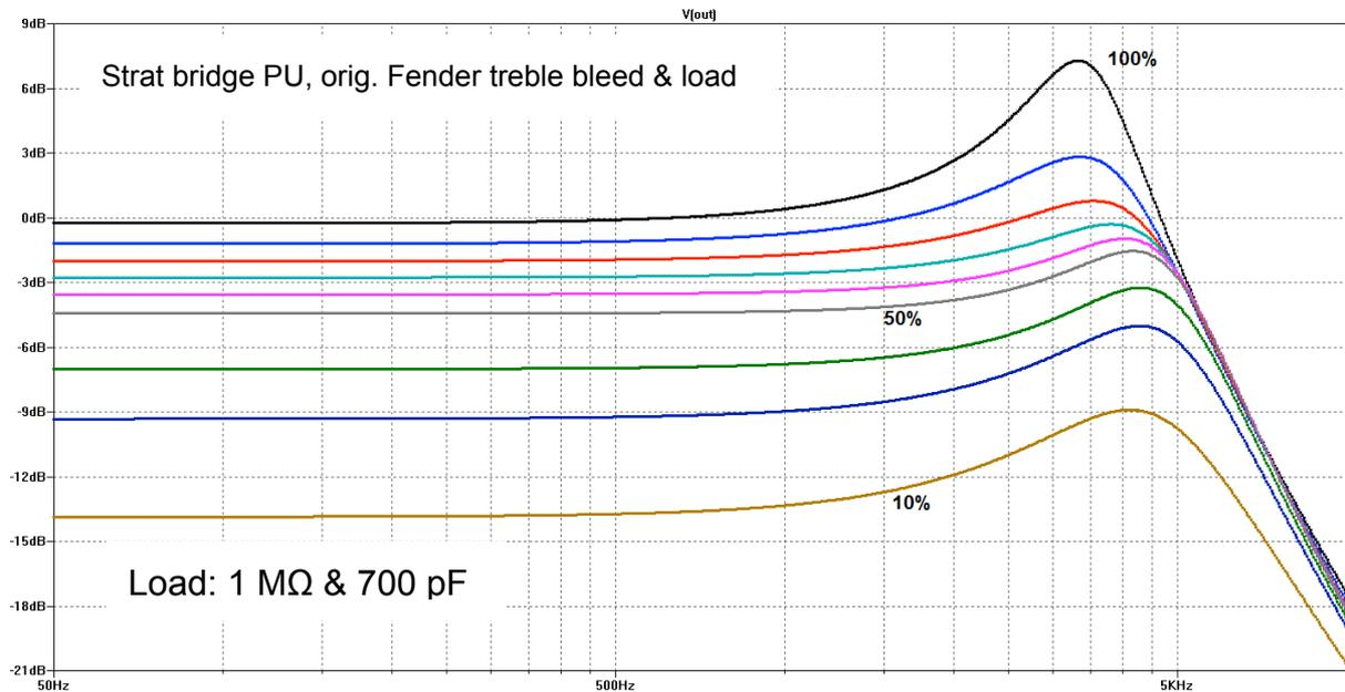
**Fig. 10:** High-impedance load; frequency responses of the Fender recommended treble-bleed arrangement (1000 pF in parallel with 150 k $\Omega$ ), at various positions of the volume control in % of the full turn angle.
