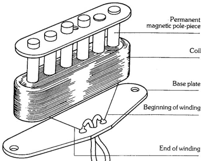
**Fig. 1:** Fender Stratocaster pickup
