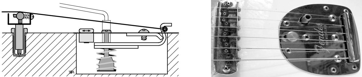
Fig. 7.120: Vibrato system of the Jazzmaster.
