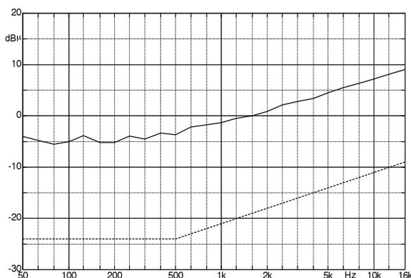
**Fig. 7.51:** 1/3<sup>rd</sup>-oct. analysis of the system noise: impedance head with charge amplifier (—); analyzer Cortex CF-100 (----). 0 dB $\mu$   $\leftrightarrow$  1  $\mu$ V.
