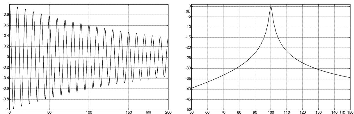
**Fig. 7.57:** Time function and spectrum of an exponentially decaying cosine-tone;  $f = 100$  Hz,  $\tau = 200$  ms.
