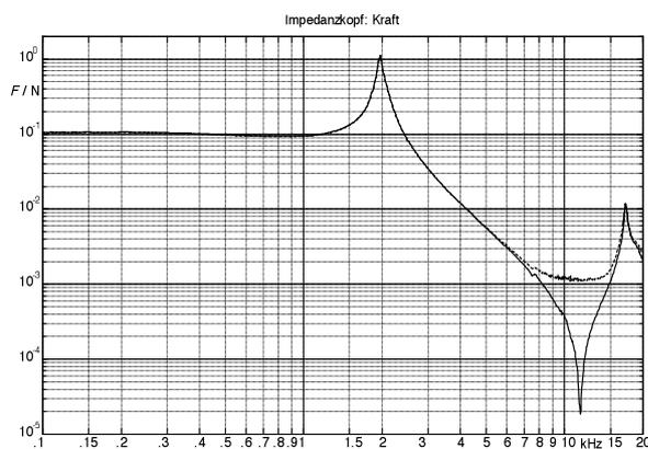
**Fig. 7.56a:** Force measurement; probe tip directed against the stone table. Without (----) and with (—) tracking filter. The force changes by 1:70000 across the frequency range; such a large dynamic range is only manageable with a selective measurement.
