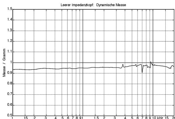
**Fig. 7.49:** Left: magnitude of the co-vibrating complex mass  $\underline{F}/\underline{q}$  of the impedance head. Below: Force-flow-diagram of the equivalent systems. “Leerer Impedanzkopf” = impedance head by itself; “Dynamische Masse” = dynamic mass.
