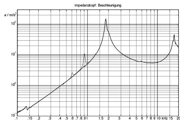
**Fig. 7.56 b:** Acceleration measurement, as given in Fig. 7.6.8a. Without (----) and with (—) tracking filter. At 600Hz and 900Hz, non-linearities excite the 1800-Hz-resonance.
