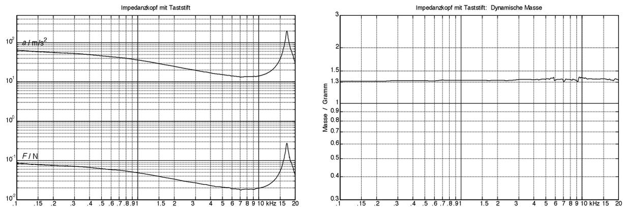
**Fig. 7.52:** Mechanical no-load condition: force and acceleration (left); dynamic mass (right);  $U_{\text{Shaker}} = 2 V_{\text{eff}}$ . “Impedanzkopf mit Taststift = impedance head including tracer pin; “Dynamische Masse” = dynamic mass
