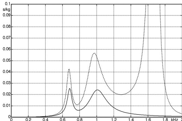
**Fig. 7.50:** Conductance without (—) and with (----) 2 g parasitic additional mass. At 1.7 kHz, the interaction of bearing suspension and additional mass results in an additional resonance peak.
