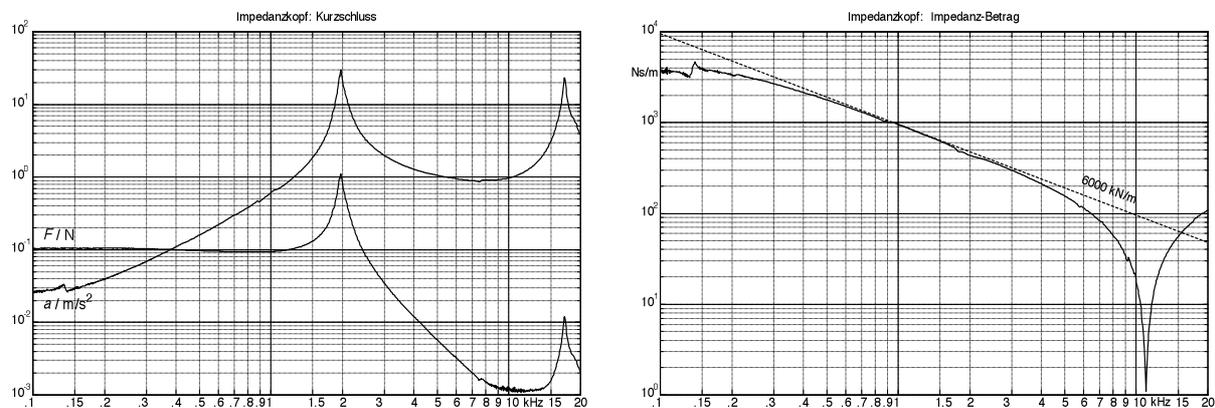
**Abb. 7.53:** Mechanical short circuit: force and acceleration (left, broadband), magnitude of the impedance (right, frequency-selective);  $U_{\text{Shaker}} = 0,1 V_{\text{eff}}$ . “Impedanzkopf” = impedance head; “Kurzschluss” = short circuit; “Impedanz-Betrag” = magnitude of impedance
