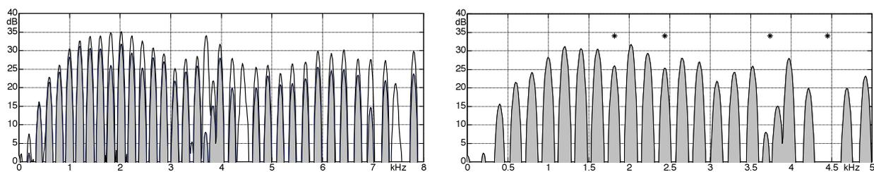
**Fig. 7.93:** Two superposed spectra, measured at a time interval of 100 ms. Frame = 21 ms, Kaiser-Window. In the right-hand picture, only the spectrum measured after 100 ms is shown. \* = areas of high damping.
