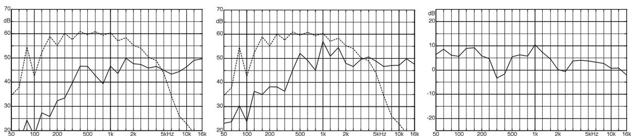
**Fig. 7.91:** 1/3<sup>rd</sup>-octave spectra of a Squier Super-Sonic: airborne sound (—), pickup voltage (----). Microphone located in the plane of the guitar body (left), microphone located in front of the guitar (center), level difference of the spectra of the airborne sound (right).
