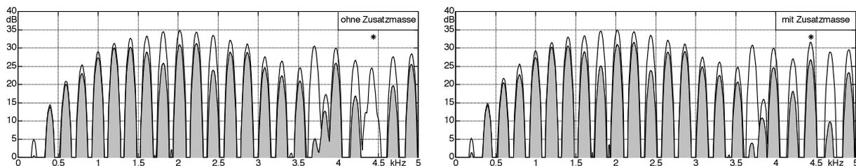
**Fig. 7.95:** Change in damping of the partial via an additional mass on the residual string. \* = 4.44 kHz.
