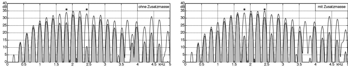
**Fig. 7.96:** Changes in the attenuation of partials by attaching an add'l mass to the bridge. \* = 1.82 / 2.44 kHz.
