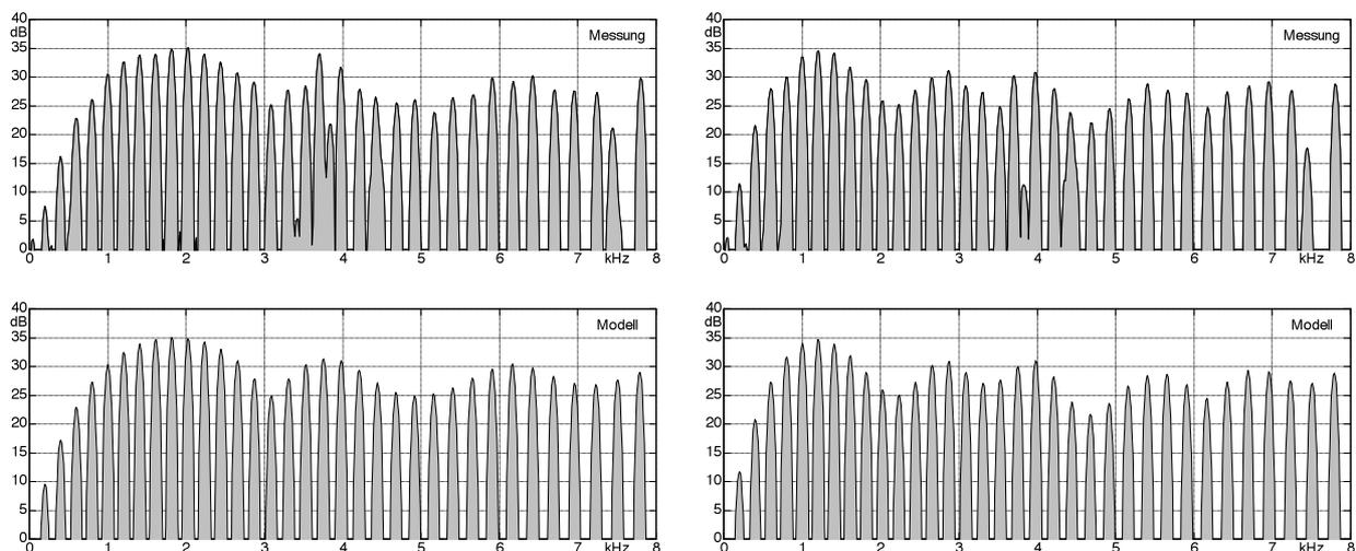
**Fig. 7.92:** Spectra of the first 21 ms after plucking the string. Two different excitations (left/right). The lower row shows the spectra calculated according to a simplified model. “Messung” = Measurement
