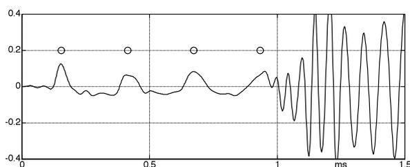
**Fig. 7.94:** Measured lateral (particle-) velocity of the string vibration. The circles mark the period of an oscillation at 3800 Hz.
