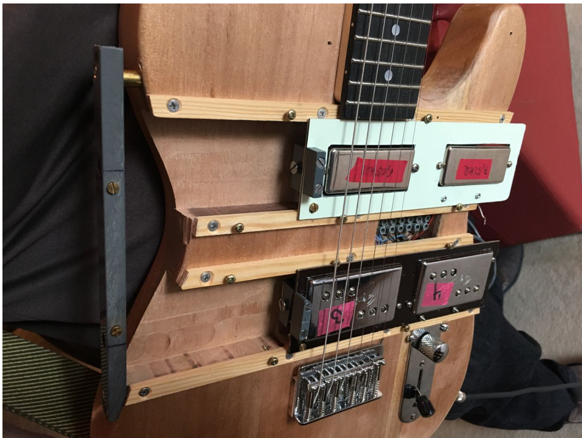
Fig. 1: Body of the "sliding pickup guitar". Both sleds are in the down position
