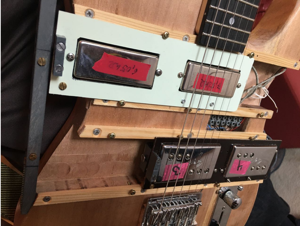
Fig. 2: Body of the "sliding pickup guitar". The sled carrying the Wide-Range Humbuckers is in the "down" position; the sled with the Firebird Mini-Humbuckers is in the "up" position
