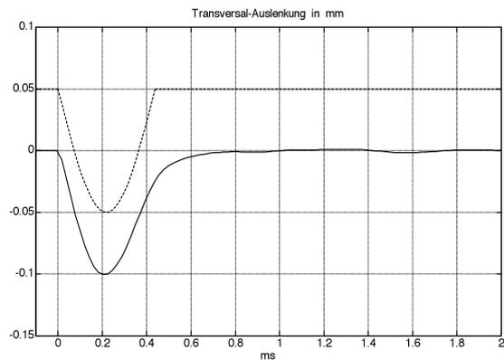
The dilatational wave remains almost invisible to the **laser-vibrometer** because the laser beam can react only to transversal but not to axial movements\*. Periodicities of  $T = 5,15$  ms are nevertheless measured – this is due to a coupling of the two wave types: the string is bent at its bearing, and here the dilatational wave returning after 5,15 ms triggers a secondary flexural wave that is visible to the laser beam.
