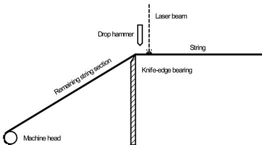
**Fig. 1.19:** Laser measuring setup (left).
