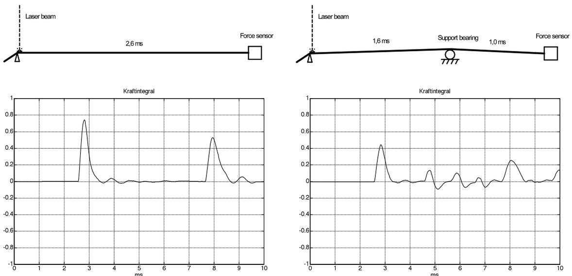
**Fig. 1.20:** Laser setup with/without support-bearing. The support-bearing separates the string length into two parts 816 cm : 511 cm. The diagrams show the temporal integral of the longitudinal string-force; the unit is Newton · millisecond (Nms). The positive sign indicates that first compression and then strain reach the sensor. “Laserstrahl” = laser beam; “Kraftsensor” = force sensor; “Kraftintegral” = force integral; “Stützlager” = support-bearing.
