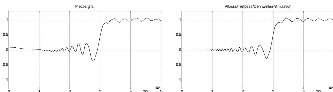
**Fig. 1.17:** Measurement (left) and dilatational-wave simulation (“Dehnwellensimulation”, right); step-excitation at mid-string at  $t = 0$ ,  $E_2$ -Saite. “Tiefpass” = low-pass.
