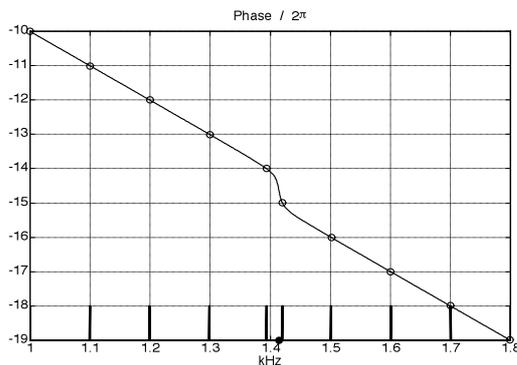
**Fig. 2.21:** Phase shift along a full travel path along the string. One string bearing is configured as a resonator resonating at 1,415 kHz. An additional natural frequency is the result of the narrow-band additional phase shift.
