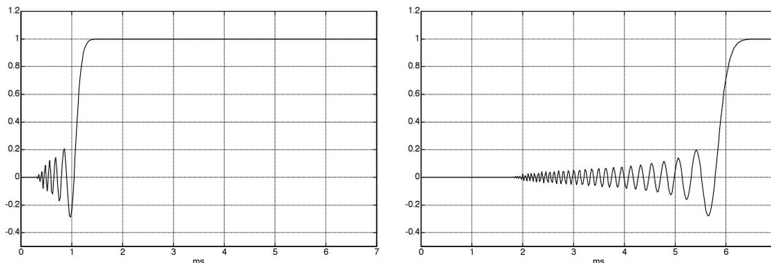
**Fig. 2.43:** Step response of a cascade of 14 (left) and 74 (right) all-pass filters. Data as in Fig. 2.42. In addition to the all-passes, a slight treble attenuation was included (*one* 1<sup>st</sup>-order low-pass at 10 kHz).
