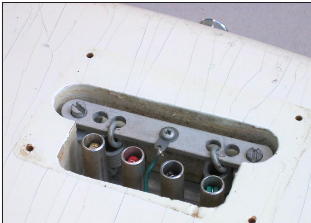
Fig. 3: The bridge unit is movable and hold by two strong springs. But there is no vibrato lever.
