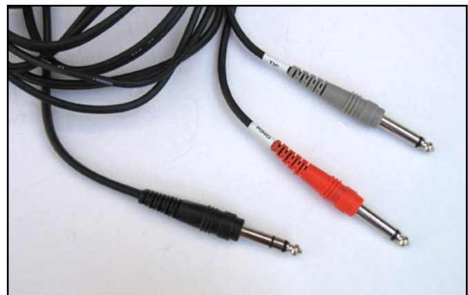
Fig. 6: A “Y” cable, with two mono plugs in one end, and a stereo plug in the other.
