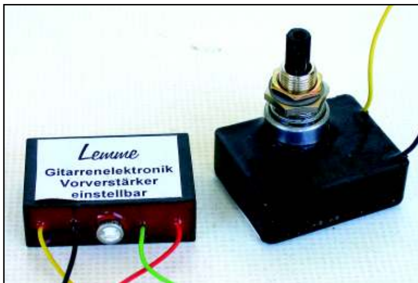
Fig. 7: Taking the low impedance pickups to their highest expression: an extremely low noise preamplifier (with active treble and bass control and passive components for midrange control- left) and the improved 'Decade' switch—exponentially graded, embedded in epoxy resin, and easily exchangeable (right).
